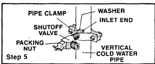
6. Slip compression nut and compression sleeve on copper tubing as shown in diagram. Insert end of tubing into outlet end squarely as far as it will go. Screw compression nut to outlet end with adjustable wrench. Do not overtighten. Turn ON main water supply and flush out tubing until water is clear. Turn OFF shutoff valve on the water pipe. You are now ready to connect other end of ¼-inch copper tubing to inlet tube or water valve on back of refrigerator.
